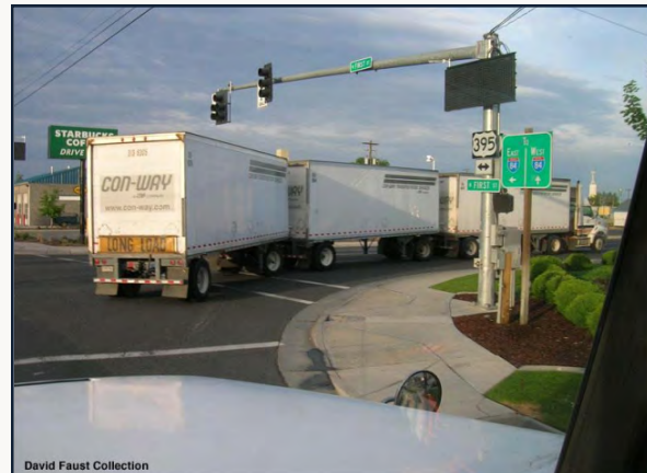
Figure 2.2: Pup Trailers: As mentioned above, pup-trailers can come in two or three 28' trailers used in line haul movements for LTL networks.
